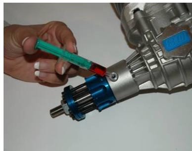
Inject 1.5ml of oil for engines to the hole as in the picture.
