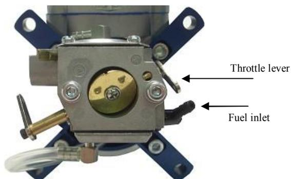
Caution! Never tight the adjusting needles by force. You can damage the touching flats for the needles. In this way damaged parts cause the carburetor is not possible to adjust and it is necessary to exchange new carburetor.
